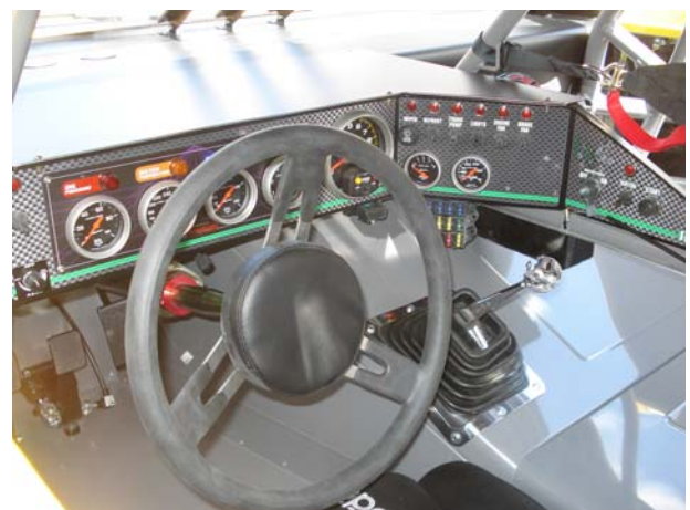
The cockpit includes gauges for oil pressure and temp, water temp, fuel pressure, fuel level and trans temp. Switches for engine and brake fans, trans pump, defrosters, tail lights, fresh air system and windshield wipers.
