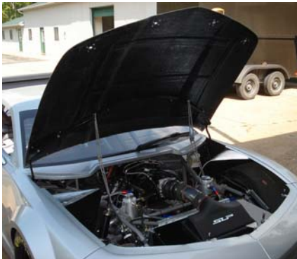
Optional Hinged hood with Schwanke LS3 Engine.
