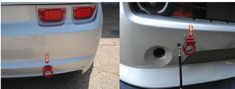
LED tail and brake lights and SCCA legal tow loops front and rear.
